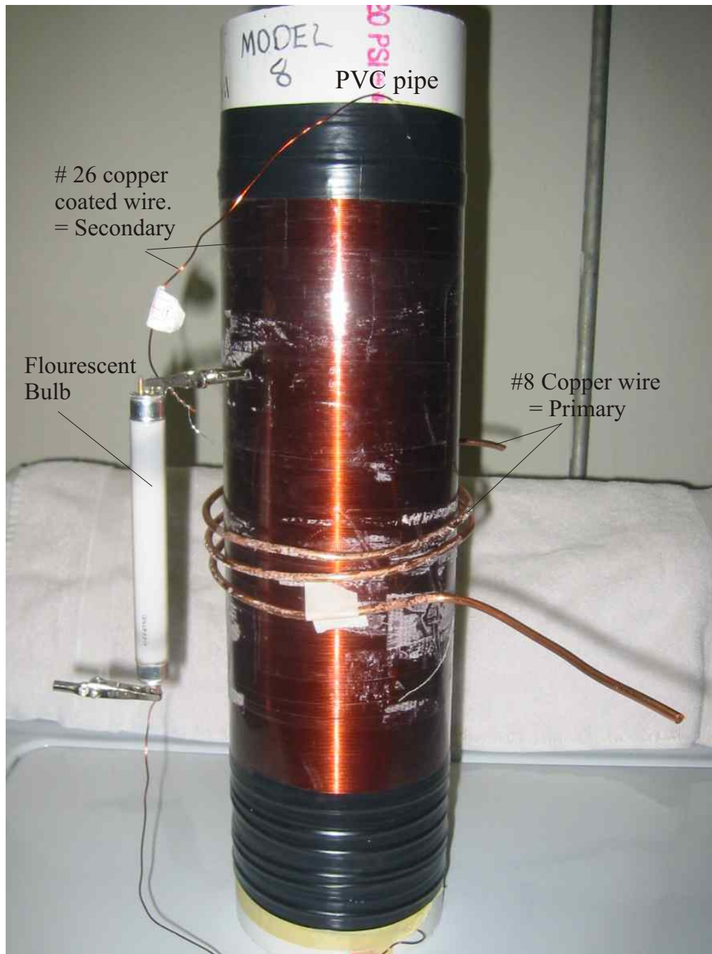
Creative Science & Research: Our Homemade Tesla Coil, Great for many high voltage and free energy experiments.
