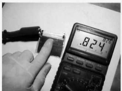
Two cells measures .824 vDC
