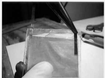
Bending back metal contacts
