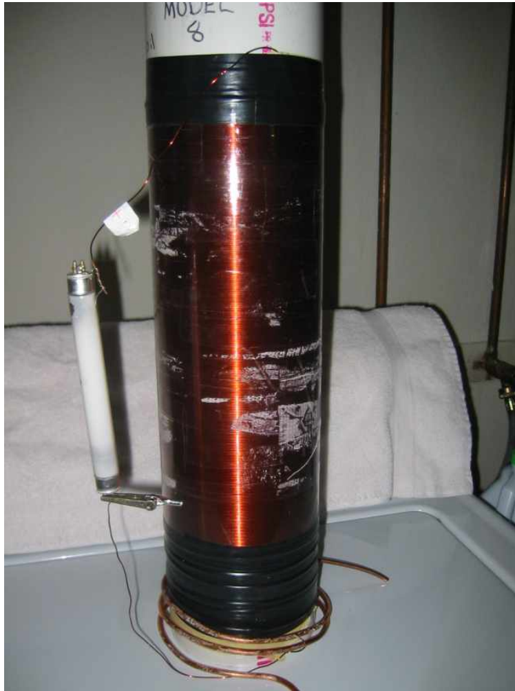
Homemade HV Tesla Coil
