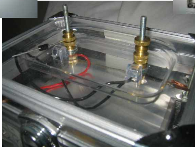
High Voltage Capacitor Terminals
